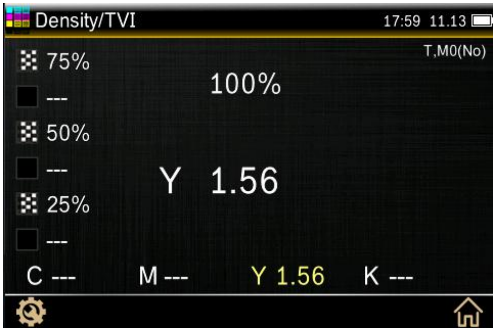
Figure 21 Density/TVI Interface Measurement Data
